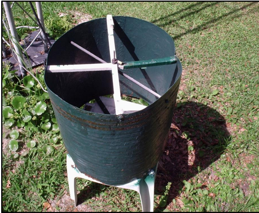
Figure 6.19 - Pat W5THT, foil wound lightweight inductor.
